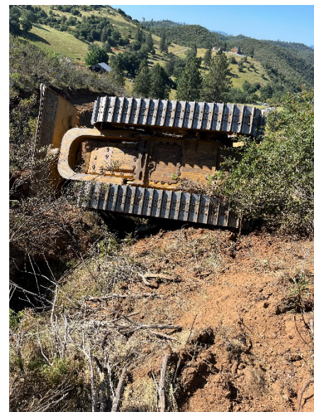
Figure 6: Bottom of bulldozer after rollover.
