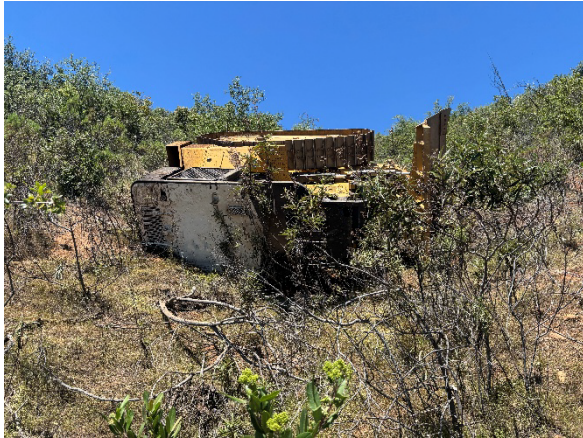
Figure 5: Top of bulldozer after rollover.
